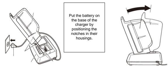
Turn the battery as shown on the picture on the left
