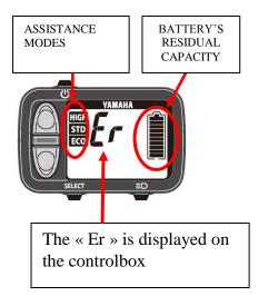
Your Axion is equipped with a selfchecking system of the assistance system. If any failure or defect of the assistance system's operation, when the controlbox is powered, the display « Er » is displayed on the controlbox. The displays for the battery's residual capacity will flash in alternance when there is something wrong with the assistance system's operation.
