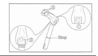
Loosen with an Allen key the fixing screws 1, 2 or 3 around 3 turns. - Set the handlebar slope
