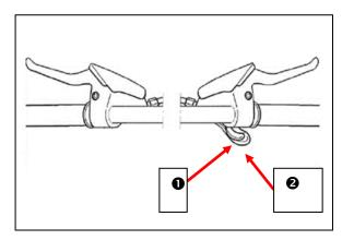
Gearshift push levers. The lever 1 is used to gear up. The lever 2 is used to gear down.'
