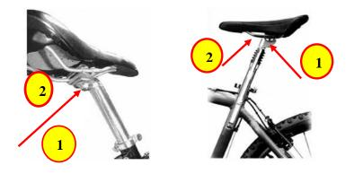
For the setting of the seat post position loosen the screw (1) and change the position of the saddle rails (2) so you are able to find the optimal use position.
