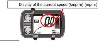
The speed is displayed in kmprh (mprhr). NOTA : If your speed is lower than 0,5Kmprhr, the displayed speed is 0,0Kmprhr.
