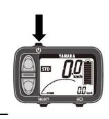
For the assistance system push the button « ON » Immediately when the controlbox is on « ON », the display of the functions is enlighted completely during the autotest of the controlbox. After the indicator is automatically positioned on « STD » and displays the available battery residual capacity.
