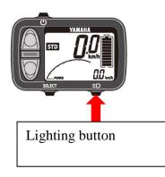
For the operation of the lighting, push on the lighting button. By pushing on the lighting button :
