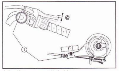
@ : Stroke : 15mm 1 : Setting's thumbwheel
