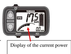
The current power display gives an estimated current power of the assistance on a scale 1 - 8. The assistance system is not in function when no display. Any increasing of the power will gradually be displayed.
